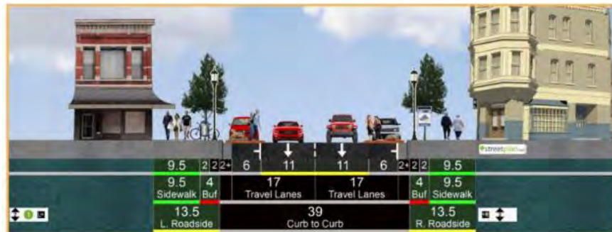
OPTION E - TWO LANE, ONE WAY TRAFFIC WITH PARALLEL PARKING BOTH SIDES & BUMPOUTS
